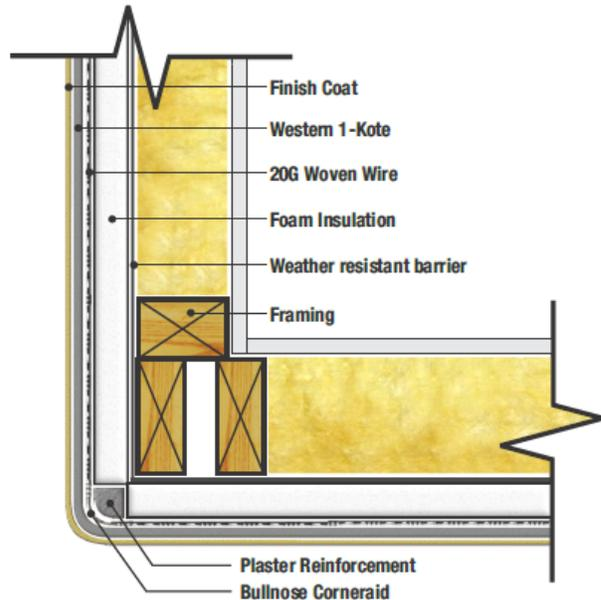
**Figure 7 - One Hour Firewall Assembly No. 1 (Table 1)**
