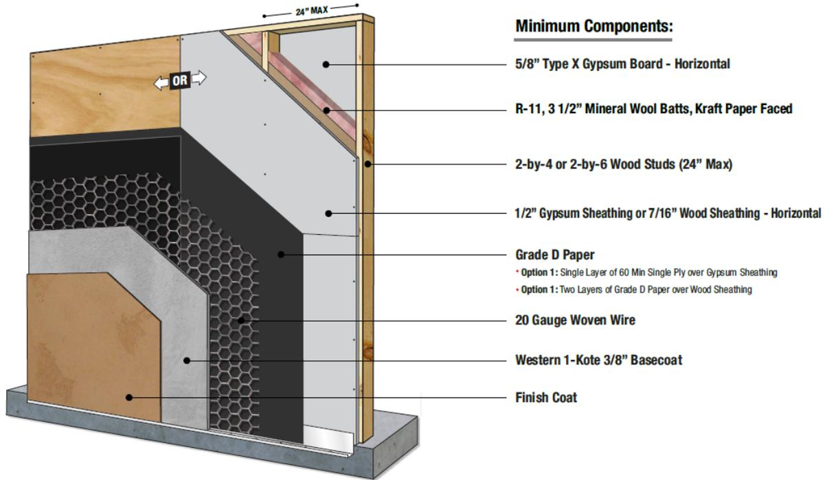
Figure 10 - One Hour Firewall Assembly No. 4 (Table 4)
