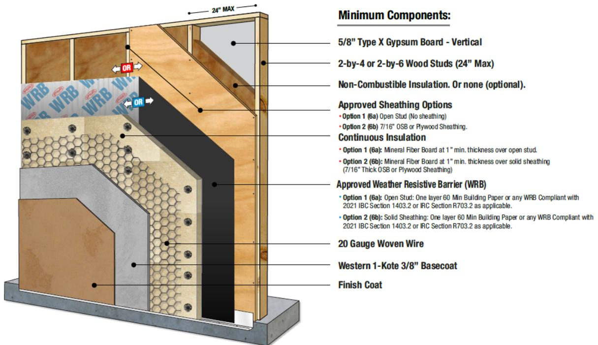
Figure 13 - NFPA 285 Assembly without Continuous Insulation (Table 6)
