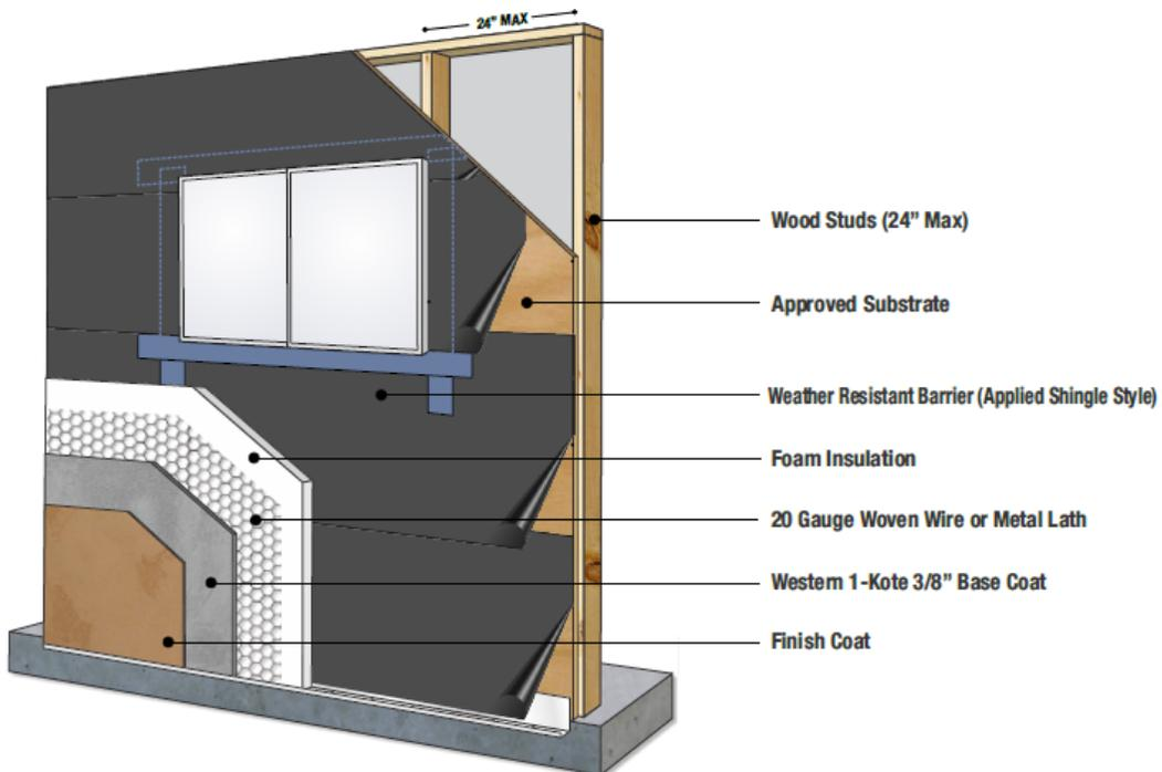
**Figure 5 - Plaster Termination at Window with Integral Flange**
