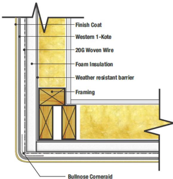
**Figure 6 c - Corner with Reinforcement**
