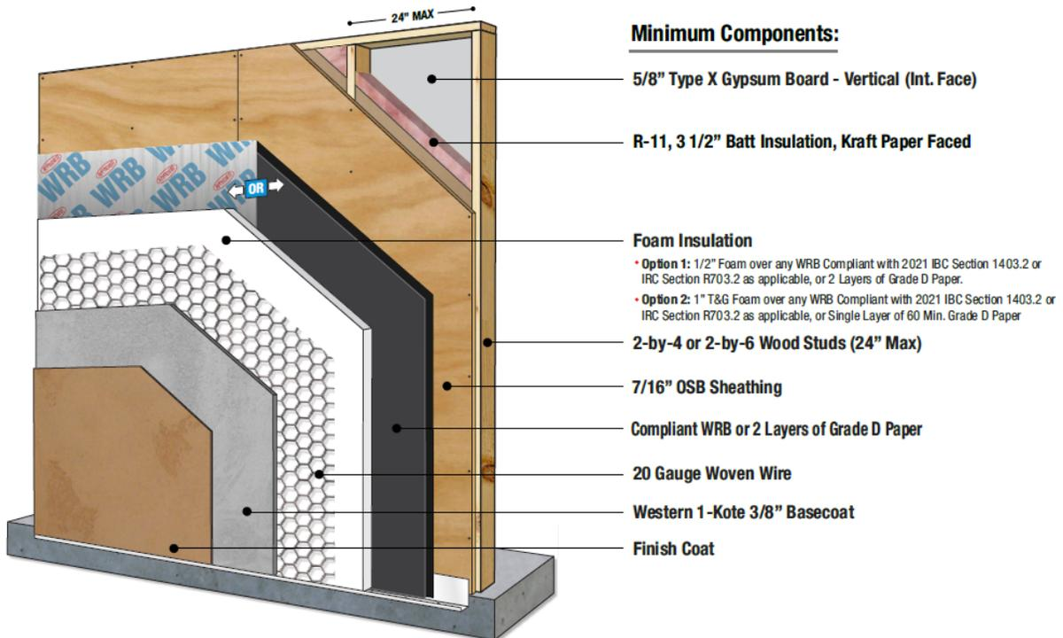
Figure 11 - One Hour Firewall Assembly No. 5
