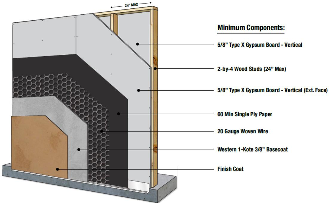
**Figure 8 - One Hour Firewall Assembly No. 2 (Table 2)**
