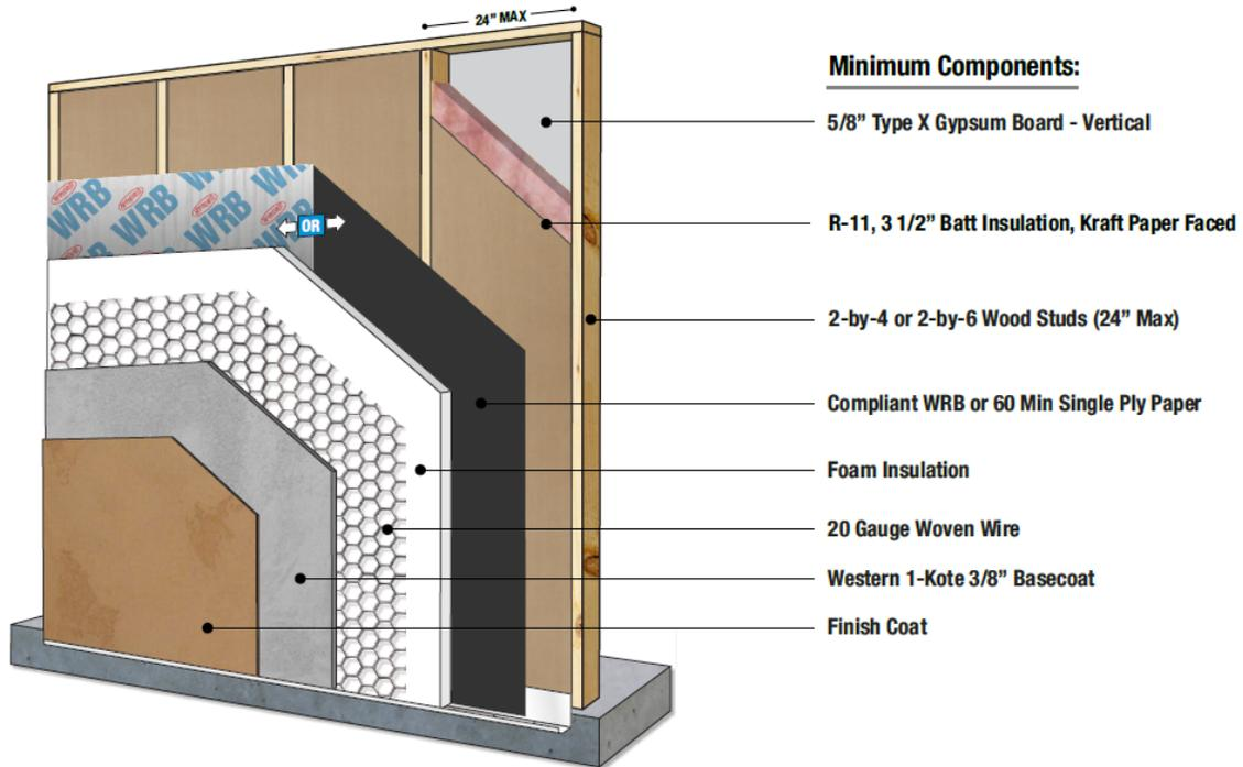
Figure 12 - One Hour Firewall Assembly No. 6
