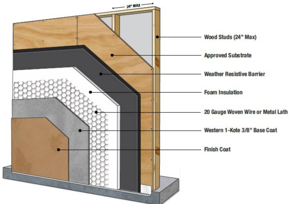
**Figure 3 - System with Unbacked Foam Plastic**
