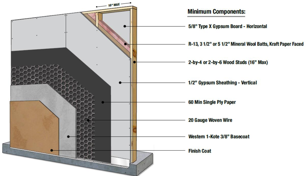
Figure 9 - One Hour Firewall Assembly No. 3 (Table 3)
